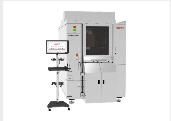
Figure 2: FIREBIRD Series thermocompression solution SOURCE: ASMPT
